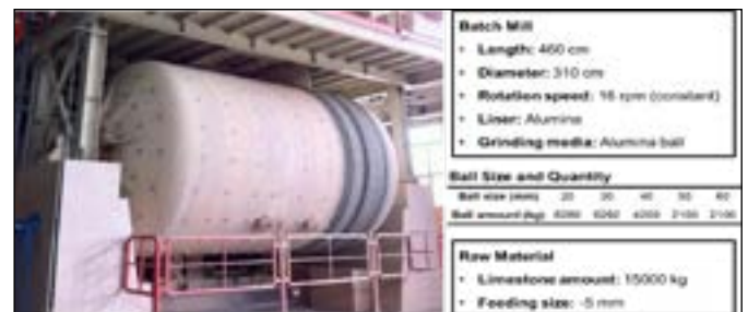
Figure 2. Representative demonstration of batch mill and wet grinding parameters
