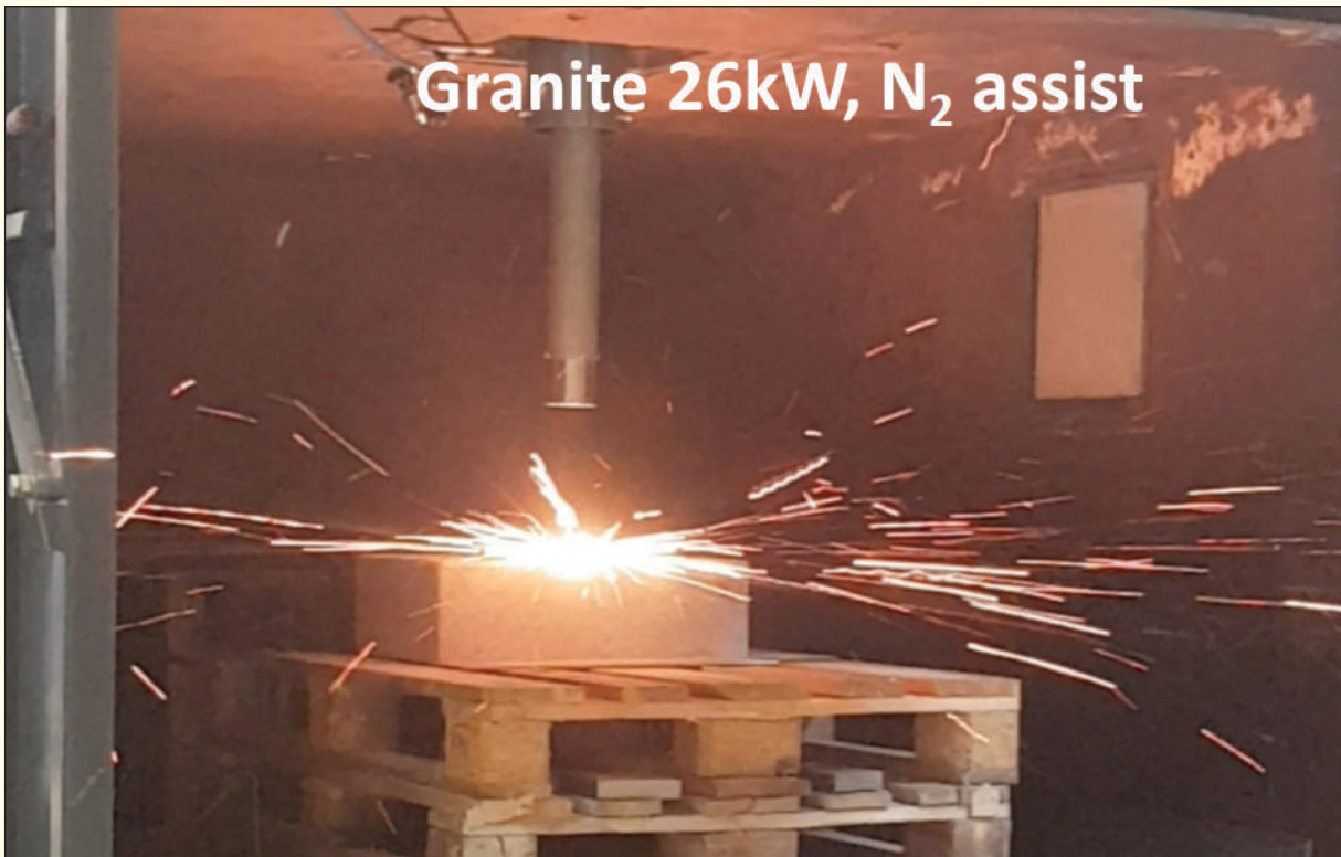
Figure 2: Experimental set up during a test with a granite slab (50x35x15 cm).
