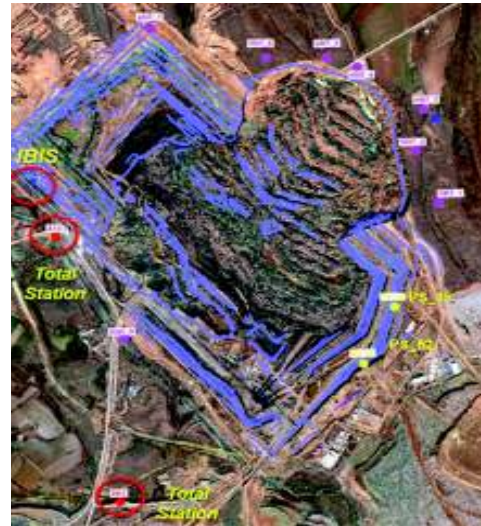
Figure 5. Planimetric view of Çollölar mine. IBIS-M wide coverage makes it possible to cover the entire area of interest from a permanent installation on the opposite side of the pit.
