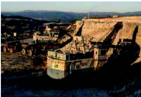
Figure 3. Excavator - truck method
