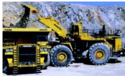
Figure 2. Komatsu WA1200 36 Tonne Mechanical drive Wheel Loader
