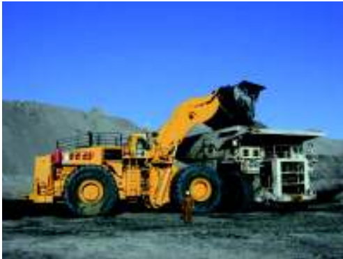
Figure 3. LeTourneau L-2350 Electric Drive 72 Tonne Wheel Loader.
