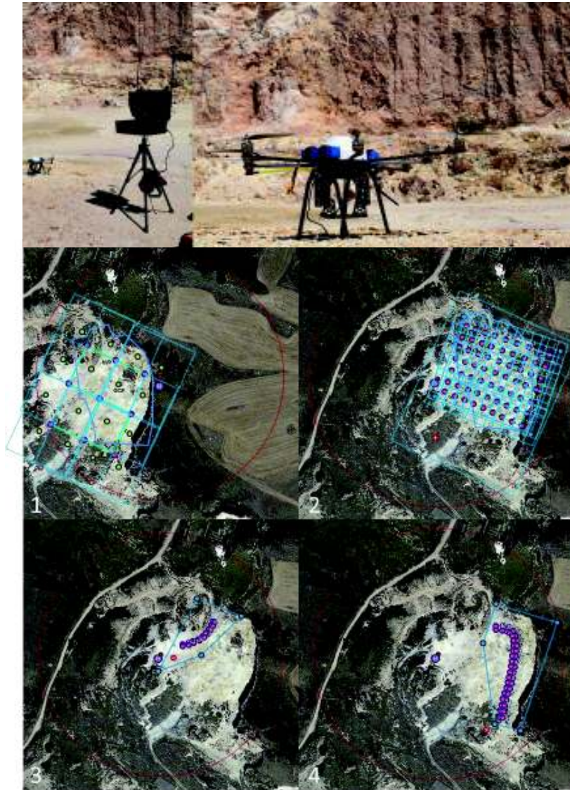
Figure 3. The UAV multirotor platform assembled with OEM electronic components (by MikroKopter HiSystems GmbH) with Ground Station control unit and waypoints of the flight plans pre-elaborated with “GeoMapTool 4.0” (by Alex Demeo) for “MikroKopterTool. 1) Preliminary flight plan, 2) Complete Nadiral flight plan and 3),4) vertical flight plans.
