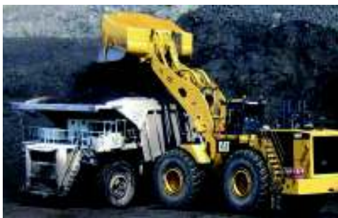
Figure 1. CAT994 35 Tonne Mechanical Drive Wheel Loader.
