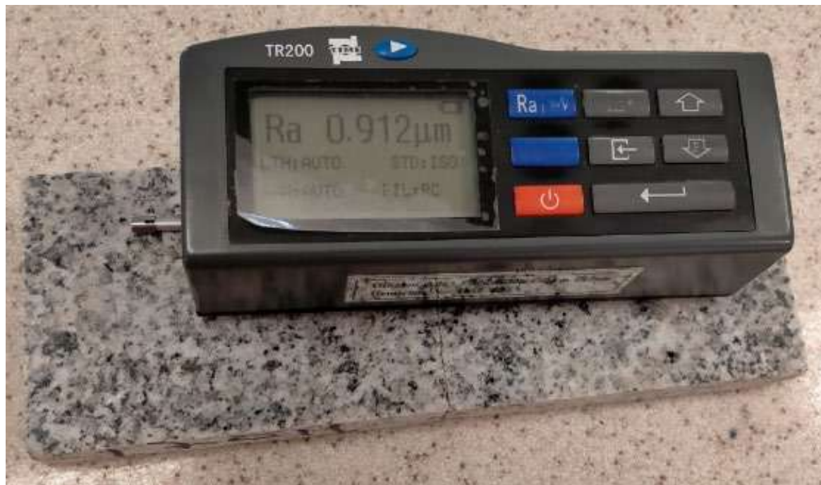
Figure 3. Roughness measuring of abraded stone surfaces
