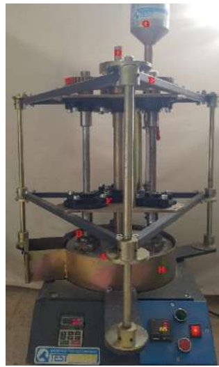
Figure 2. Abrasion test device and parts (ASTM C241)
