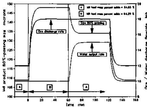
Fig 13 Overall tides of variances in mill product 80%-passing size, ore discharge rate and water output flowrate
