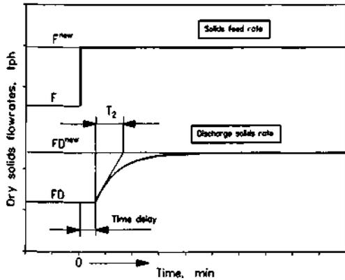
Fig. 1. Step change of dry solids input flowrate applied using an impulse manner at time  $t = 0$ , and the respective transitional process taking place in the ball mill discharge.
