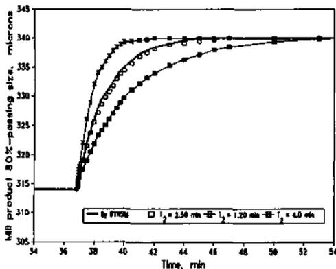
Fig. 7. Sensitivity of the response of 80%-passing size to the selection of the time constant  $T_2$ .
