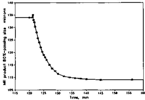
Fig 12 Dynamic response of mill product 80%-passing size to the simultaneous step decrease of water and solids feed rates
