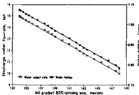
Fig. 11. Correlation between mill product 80%-passing size, and discharge water flowrate & water holdup, respectively.
