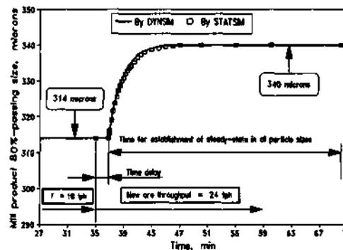
Fig. 5. Comparison between the response of 80%-passing size simulated by the DYNMIM simulator, and the same response approximated by the program STATSIM.
