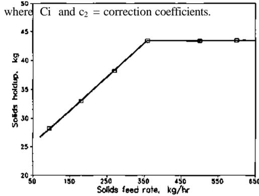
Fig. 2. Solids holdup as a function of solids feed rate.
