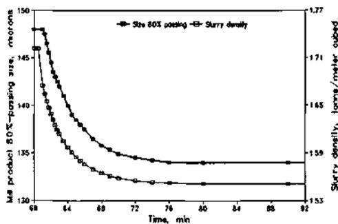
Fig. 10. Dynamic response of the 80%-passing size along with the time-dependent change of pulp density after the step increase of input water flowrate.
