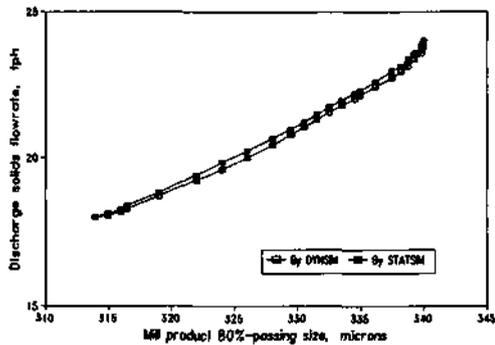
Fig. 6. Comparison of relationships obtained by the two simulators between the discharge solids flowrate and 80%-passing size in the mill product.
