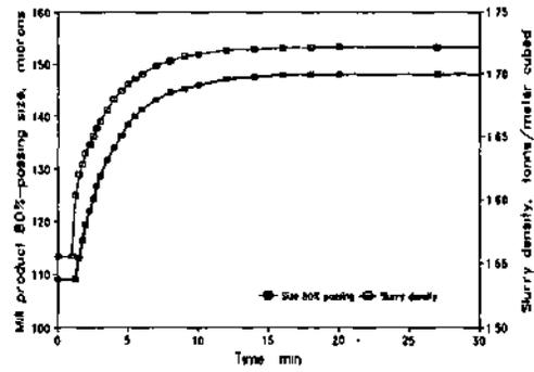
Fig 8 Dynamic behaviour of the 80%-passing size along with the time-dependent change of pulp density after the step increase of input solids flowrate
