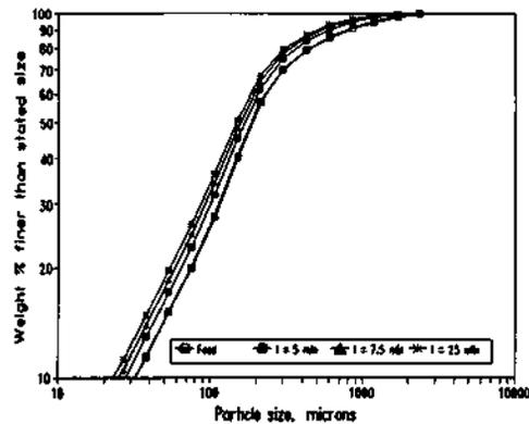
Fig. 3. Size distributions in the mill discharge at given times till attainment of steady-state.
