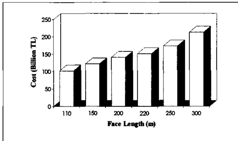
Figure 11. Total cost of conventional faces vs face length
