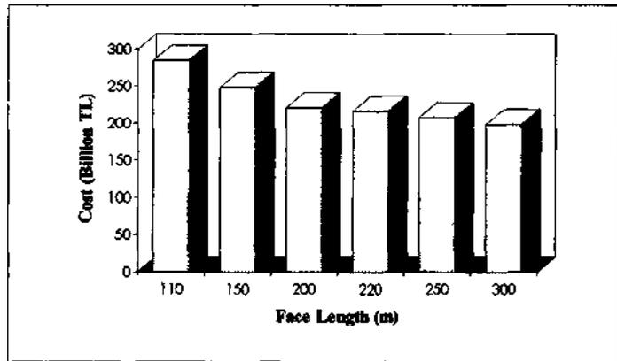
Figure 9 Total cost of face moves vs face length
