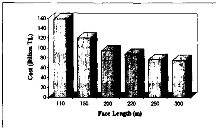
Figure 7. Total cost of road maintenance vs face length
