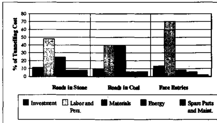
Figure 6. Cost distribution of driving roads of three distinct types
