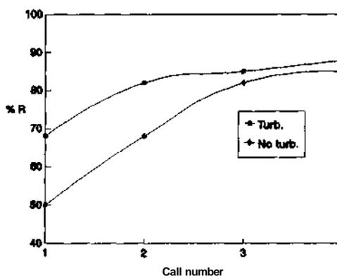
Figure 7. Effect of conditioning on copper sulfide flotation recovery and kinetics at pilot plant.
