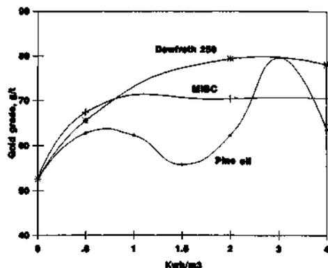
Figure 3 Effect of shear energy on gold concentrate grade for different frothers 120 g/t amyloxanthate as collector
