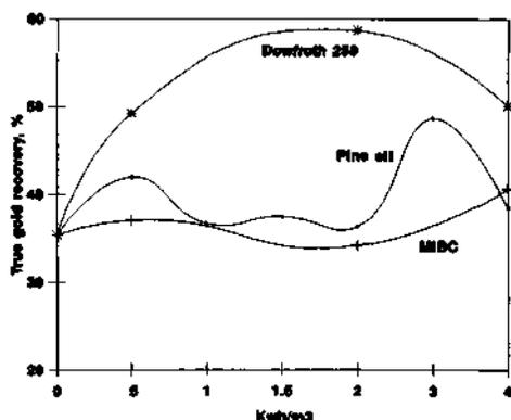
Figure 4 Effect of shear conditioning energy on gold true flotation recovery (Rt) for three different frothers 120 g/t amyloxanthate as collector
