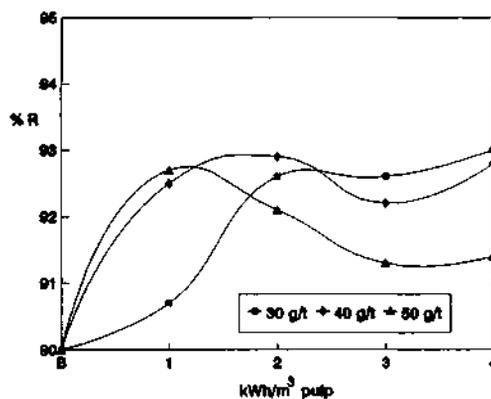
Figure 5 Effect of shear energy and collector concentration on copper sulphide flotation recovery B = Blank test, without conditioning
