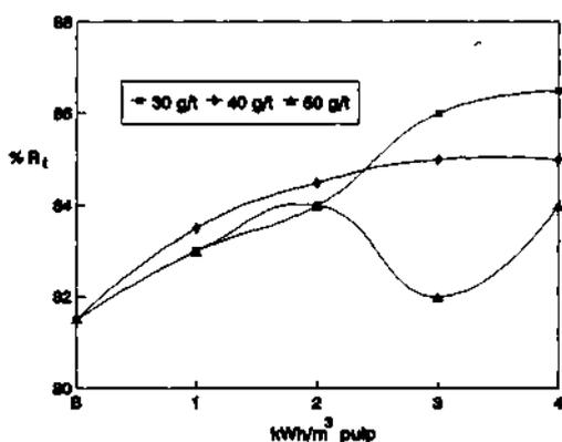
Figure 6. Effect of shear energy on copper sulphide "true" flotation recovery. B = Blank test.
