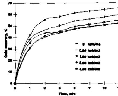
Figure 1 Flotation kinetics of gold particles as a function of the shear energy Pine oil, 72 g/t as frother and 120 g/t amyl xanthate as collector
