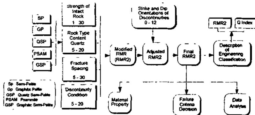
Figure 4 Rock Mass Characterisation using the RMR2.
