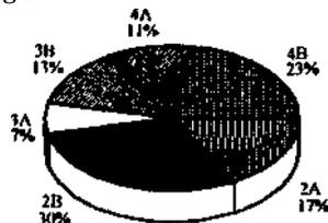
Figure 2. Distribution of rock classes encountered in exploration adit at Curnghinalt.
