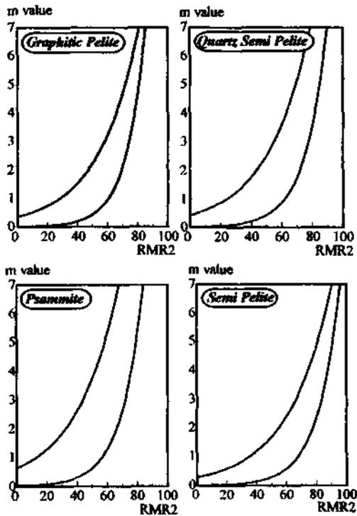
Figure 8 m value versus RMR2 for rock masses.
