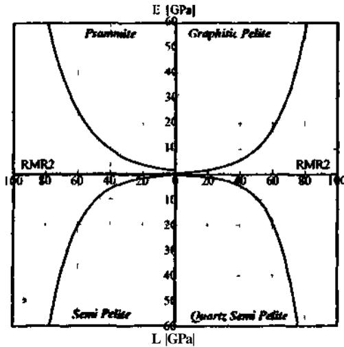
Figure 6. Elastic characteristics of rock masses.
