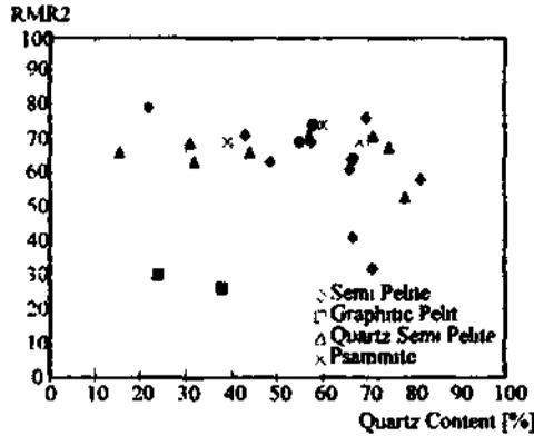
Figure 5. RMR2 versus Quartz content for various rock types at Currighinalt.
