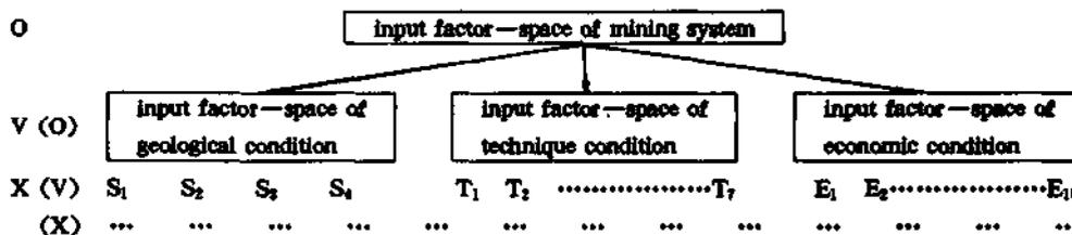
fig. 2 tree structure of mining factor—space
