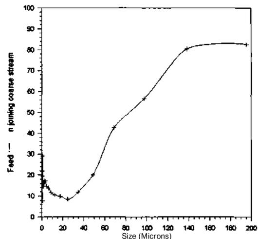
Figure 5 The Nuh Cement plant's Sepax separator performance curve
