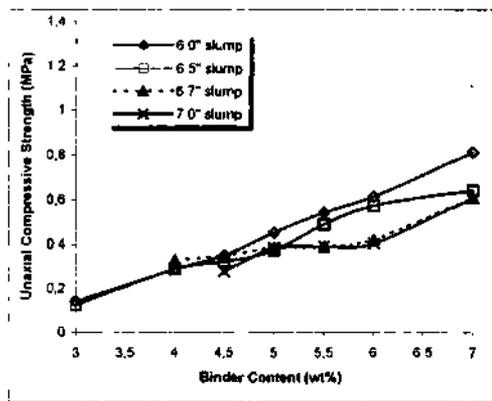
Figure 11. UCS test results for paste backfill sample B at 28 curing period.
