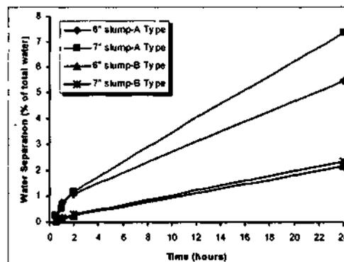
Figure 5. Water separation vs time for tailings A and B.
