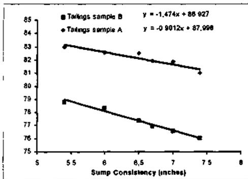
Figure 4. Solids content vs slump for ladings A and B.
