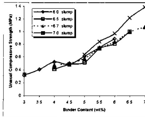
Figure 10 UCS test results for paste backfill sample A at 28 curing period
